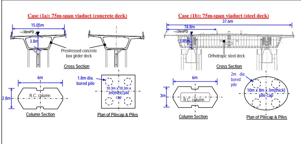
Figure 3: Bridgeforms considered in the case study (Cont'd)
