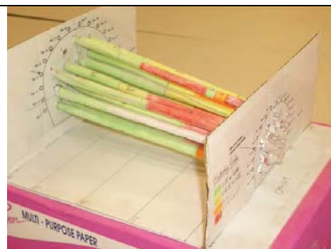
Figure 3b – 3-D models of a rock/soil interface based on logging of cuttings from drillholes for pre-reinforcement and grouting (models by Gammon Construction Ltd)
